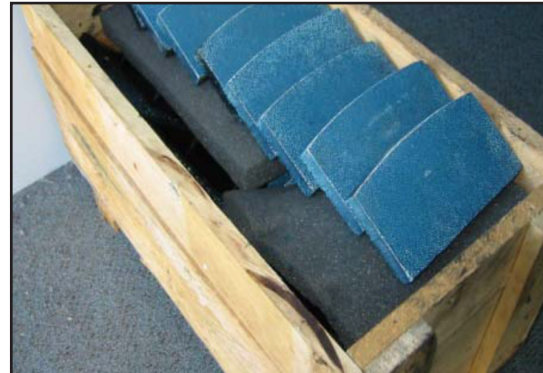
ARC molded abrasion resistant product on new blades
